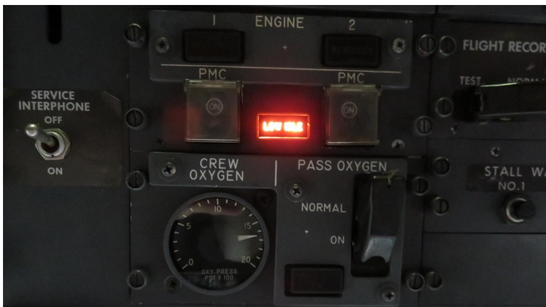
Figure 2: LOW IDLE warning for both engines, located on the overhead panel.
