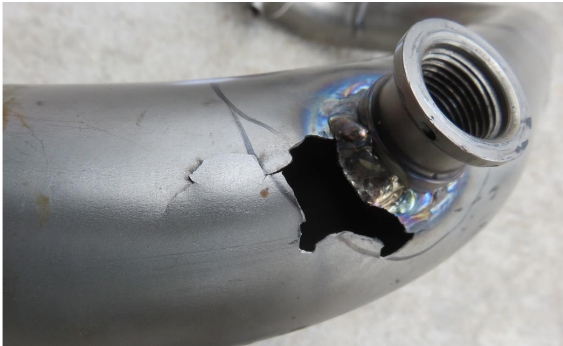
Figure 6: Damage to the Aircon Bay Compressor Outlet Duct (left air-conditioning pack).
